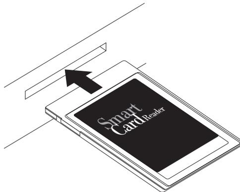
*Figure 1. Smart card installation*
