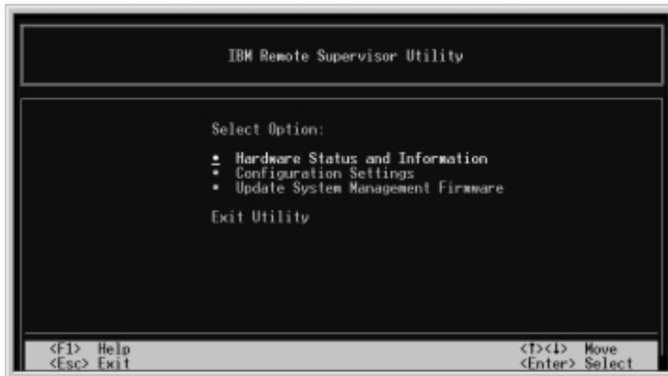
4. Use the Up Arrow and Down Arrow keys (N and N) to select **Update System Management Firmware**; then, press Enter. A warning window opens.
