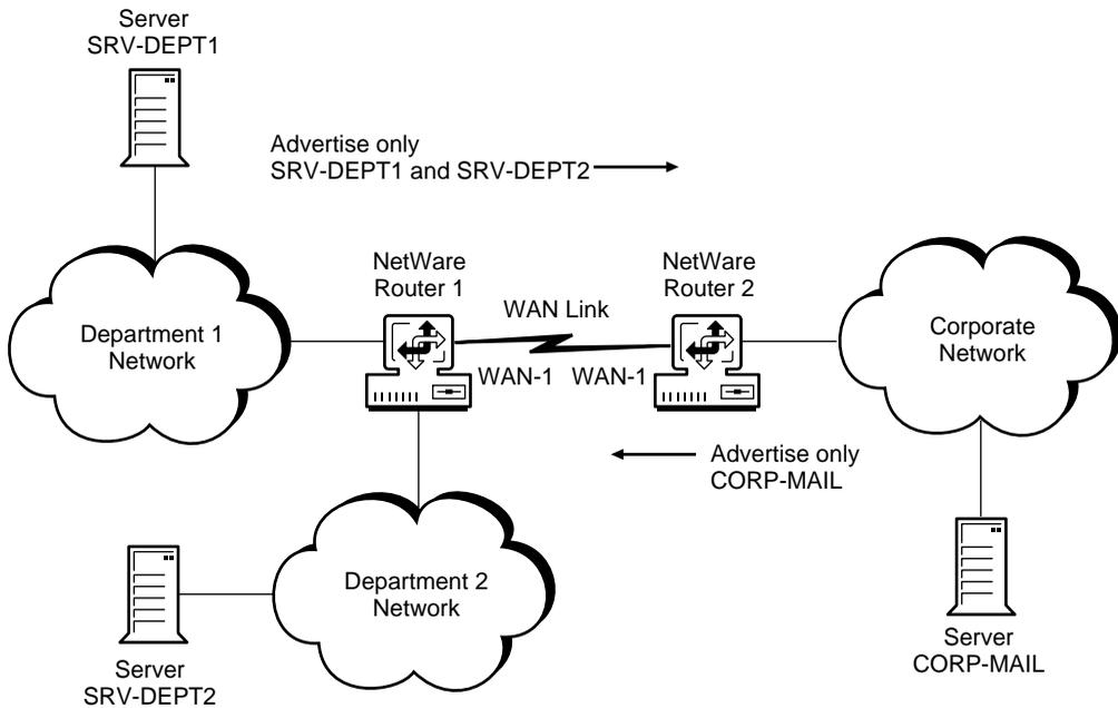
To minimize the load on the WAN link, an IPX SAP filter is configured on Router 1 and Router 2. This filter cuts down the periodic service information updates across the WAN link by advertising only a few selected servers. The clients across the WAN link can access the servers on the other network by first attaching to these selected servers.
