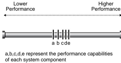
Note that all components in a well-designed system are within the same range of performance. But in this case, a less than optimum component is cost effective. The components are so closely matched that upgrading the lower-end component *a* would not increase performance enough to make it worth the cost.
