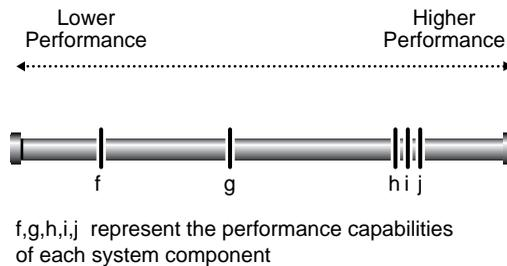
In this system, components *f* and *g* have performance characteristics that are considerably inferior to components *h*, *i*, and *j*. With component *f* as the bottleneck, components *h*, *i*, *j*, and even *g* are constrained by *f* so that they run much more slowly than their designs would otherwise permit. In this system, the bottleneck is significantly hampering the system's performance.
