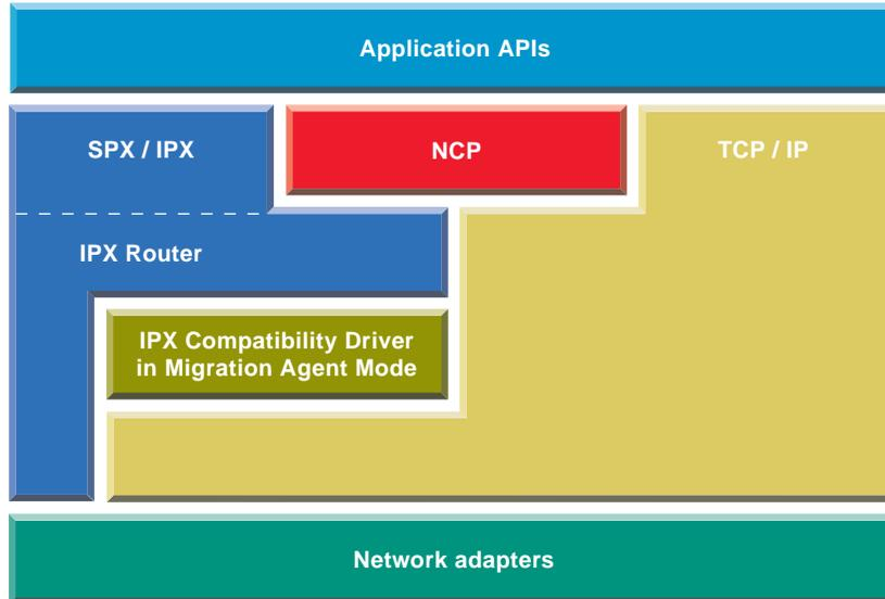
Notice that the MA makes use of the IPX router present in the IPX stack to route packets between the CMD network and the IPX networks.
