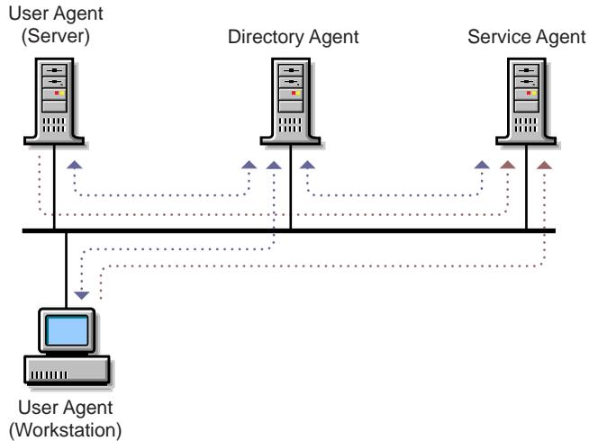
Once the application has registered with the SLP User agent, it can look up a service or get a list of services and read the attributes of a service, using either blocking calls or synchronous calls. In the IP environment, this information is pulled out of the Directory agent and put into NDS so that users and administrators can know what services are available in a local area, provided the proper security rights are granted.
