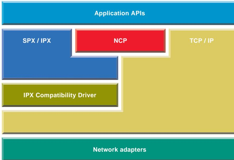
The IPX stack is loaded on systems installed with IP to give those systems the ability to execute IPX applications and to connect with IPX systems through a Migration Agent.
