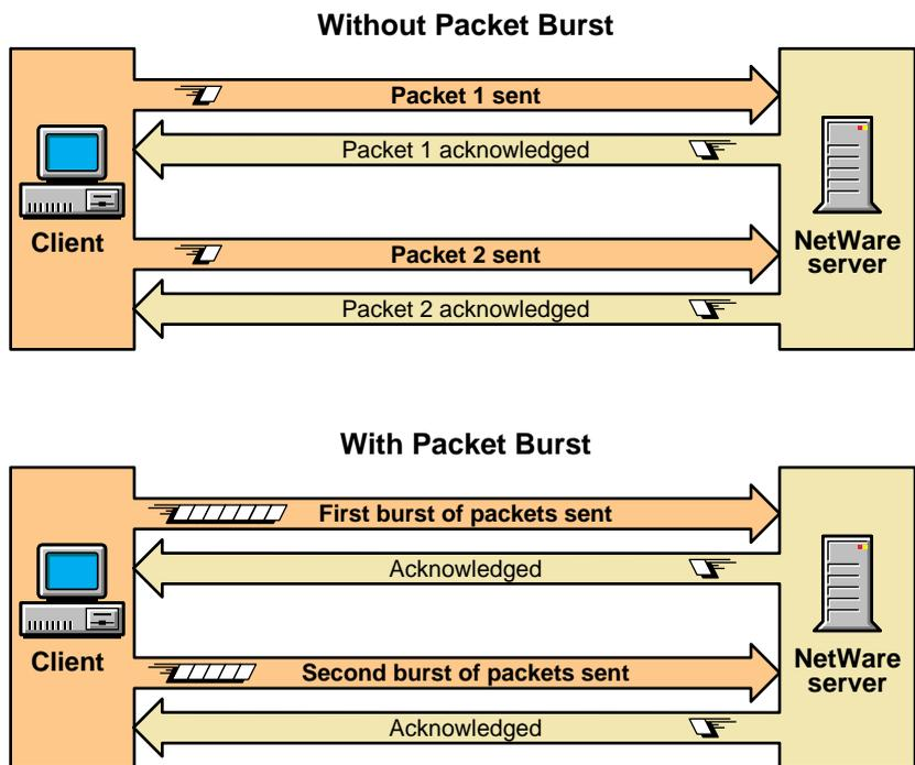
By allowing multiple packets to be acknowledged, Packet Burst protocol reduces network traffic.
