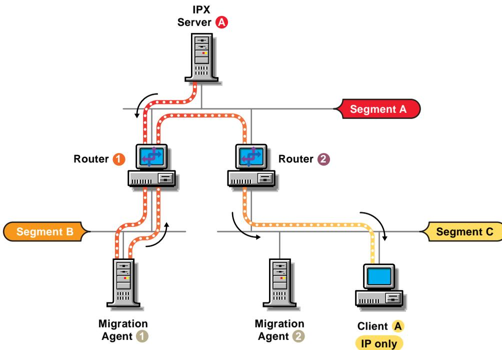
The problem presented here could be solved by placing a Migration Agent in Segment A as shown in the following figure. The Migration Server would then present to Server A the best route to the CMD network and the packets from Server A to Client A would follow the path shown by the broken line.
