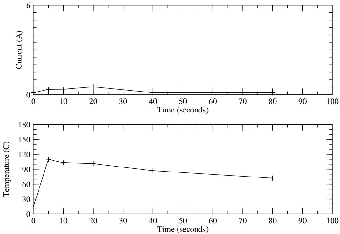
**Figure 4:** Cornichon pickle: current and temperature vs. time
