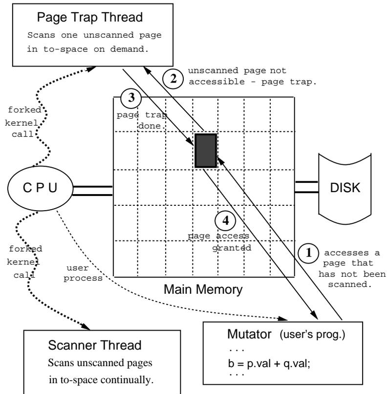
**Figure 1-2:** Appel, Ellis and Li's Incremental Collector
