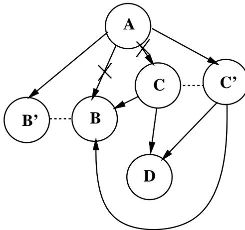
Scanning A forwards B and C to B' and C', respectively.
