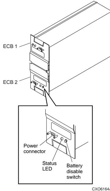
1. Press the battery disable switch (one for each battery), which is the small button labeled SHUT OFF next to the flashing status LED on the ECB and hold it in for approximately 2 seconds. The cache LED flashes once, then shuts off.
