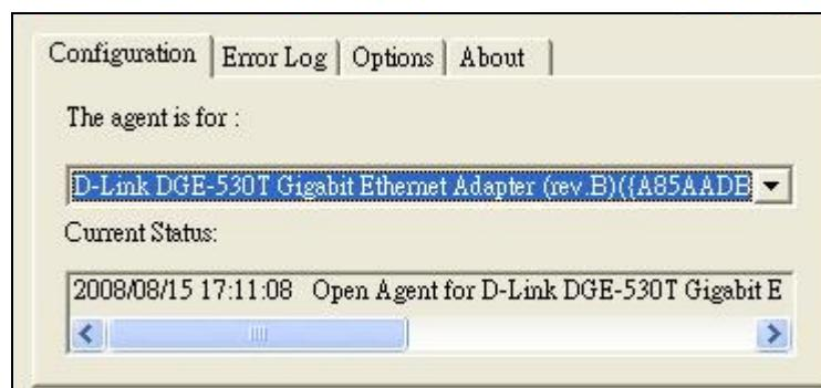
The Configuration tab has two fields. The first field, “The agent is for”, allows the user to choose an Ethernet card to configure, from a pull down menu. The “Current Status” is a read-only field which displays the most recent action made by the Ethernet card.
