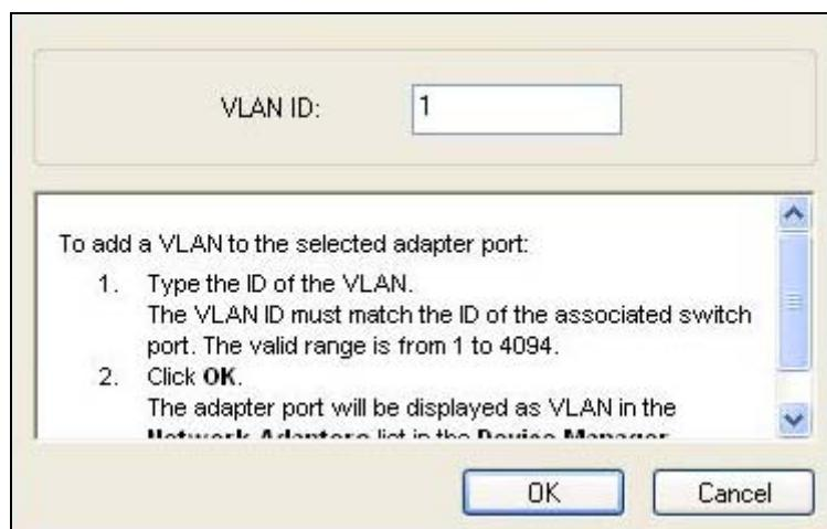
To set the VLAN, first enter a VLAN ID and then click **OK**. Available VLAN IDs are usually between 1 and 4094. The user can configure up to 64 VLAN settings for this device.
