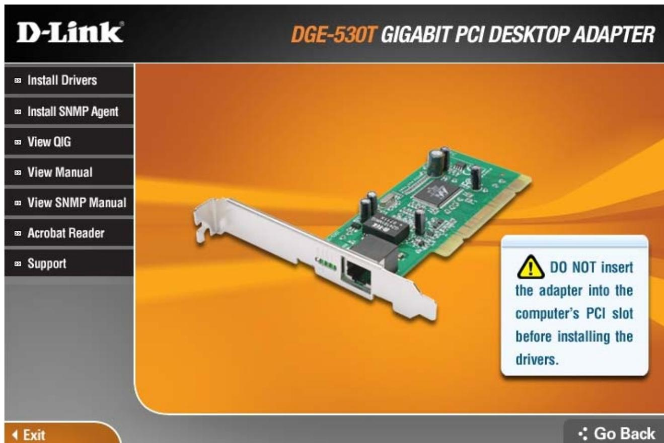
The CD included with your DGE-530T is designed to make installation of necessary software a painless and trouble-free process. Simply click on the “Install Drivers” link and an Installation Wizard will guide you through the process, no matter which operating system you’re running. Your DGE-530T will be installed successfully in just a few moments, allowing you to enjoy the many advantages of joining an Ethernet LAN.
