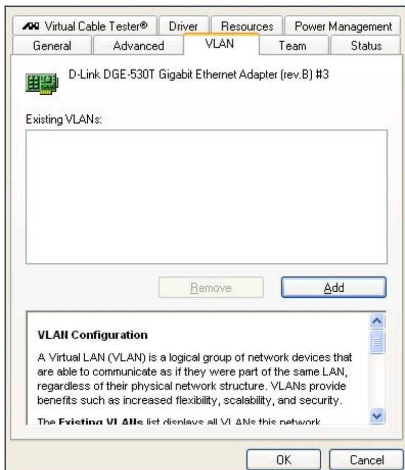
To add a VLAN setting to this window, click the **Add** button at the bottom of this window, which will open the following configuration window.
