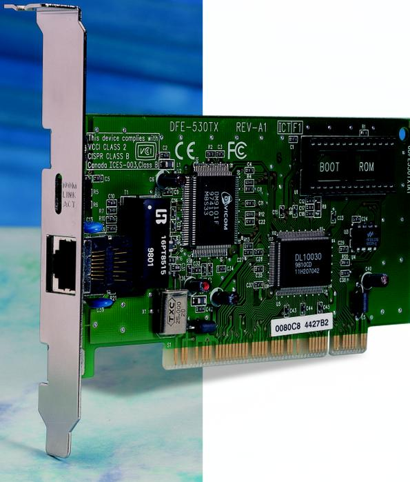
DFE-530TX Fast Ethernet adapter is equipped with an auto-negotiate 10/100Mbps NWay interface. It plugs into a desktop PC's PCI expansion bus slot to run in 10BASE-T or 100BASE-TX mode, half or full duplex.
