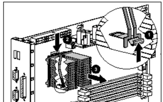
Figure 5: Processor Removal
