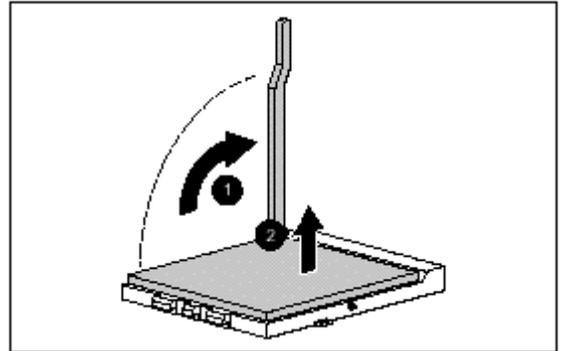
Figure 6: Processor Replacement
