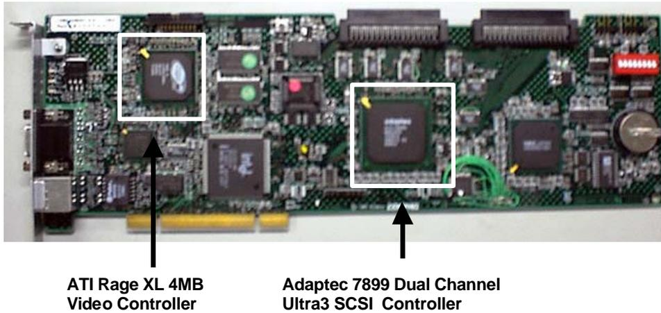
Figure 2 illustrates the new features found on the ProLiant ML350 system board:
