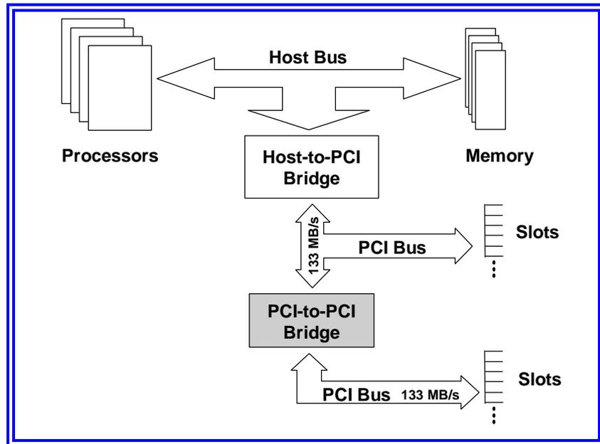
Figure 5: PCI-to-PCI bridge architecture.
