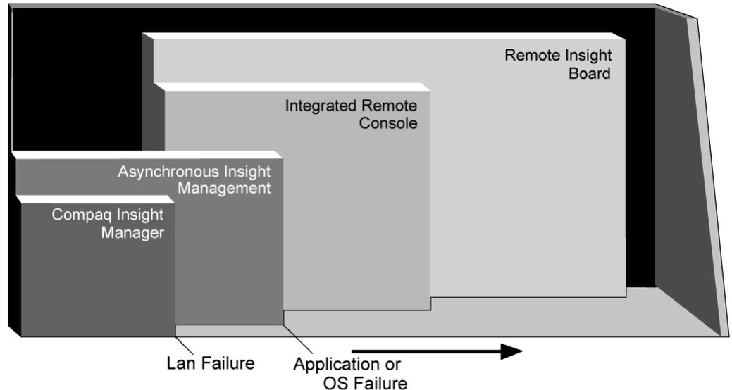
Figure 6: When an OS failure occurs, the hardware-based IRC and Remote Insight tools are required because OS-based tools such as Insight Manager and Asynchronous Insight Management can no longer function. The arrow indicates increasing severity of failure.
