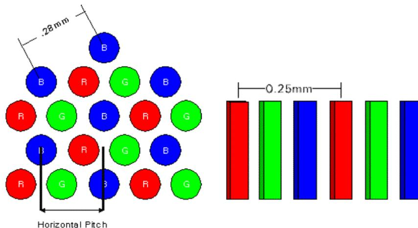
**In aperture grille CRTs, the pitch is measured either on the phosphor (stripe pitch) or is measured on the wire, when it is defined as the grille pitch.**
