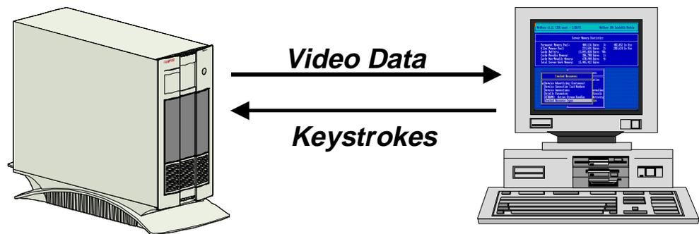
Figure 2: Graphic representation of IRC remote console capability.
