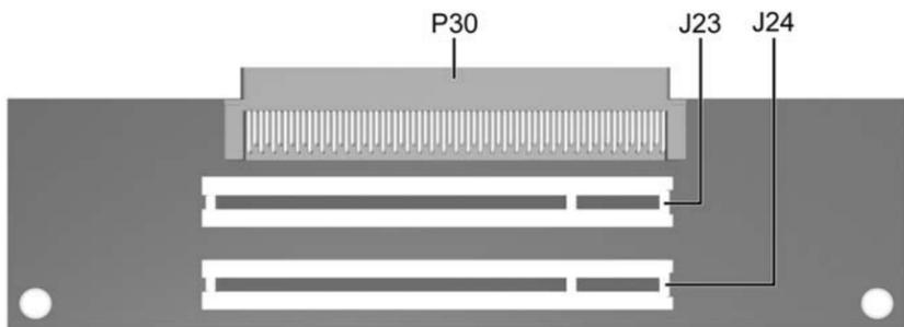
**PCI Extender Card Connectors and Jumpers**
