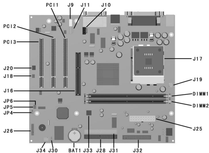
**System Board Connectors and Jumpers, Type 1 Chassis**
