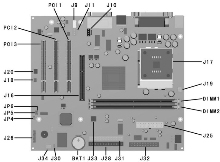
**System Board Connectors and Jumpers, Type 1 System Board**
