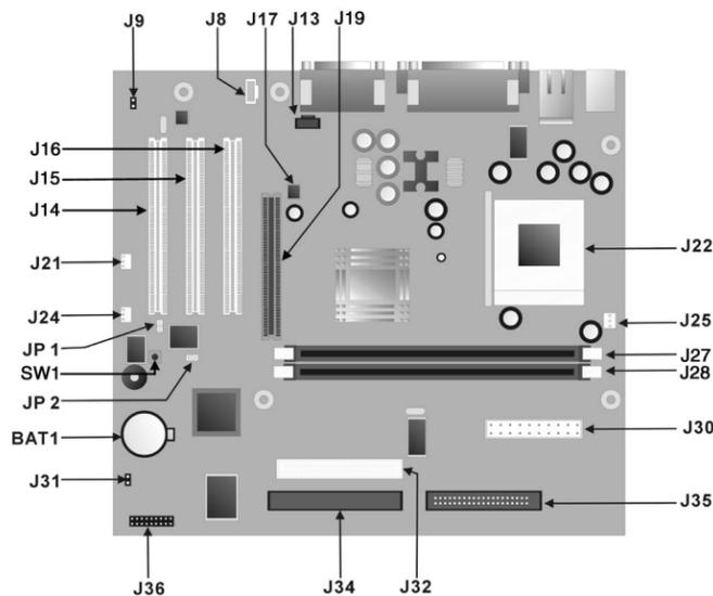
**System Board Connectors and Jumpers, Type 2 System Board**
