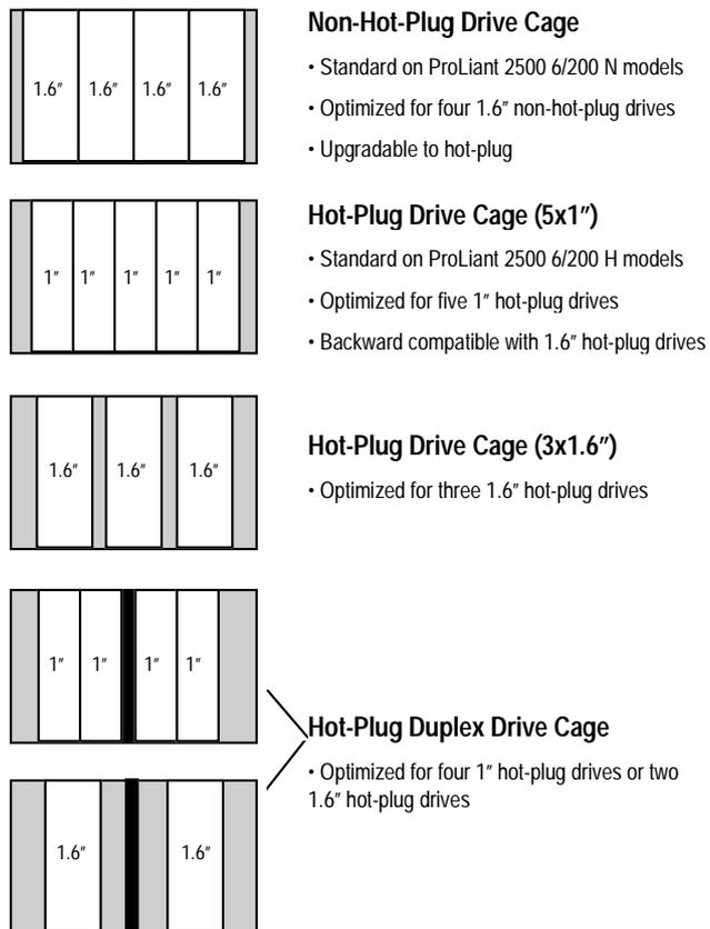
Figure 9. Available drive cage configurations for the Compaq ProLiant 2500 Server.
