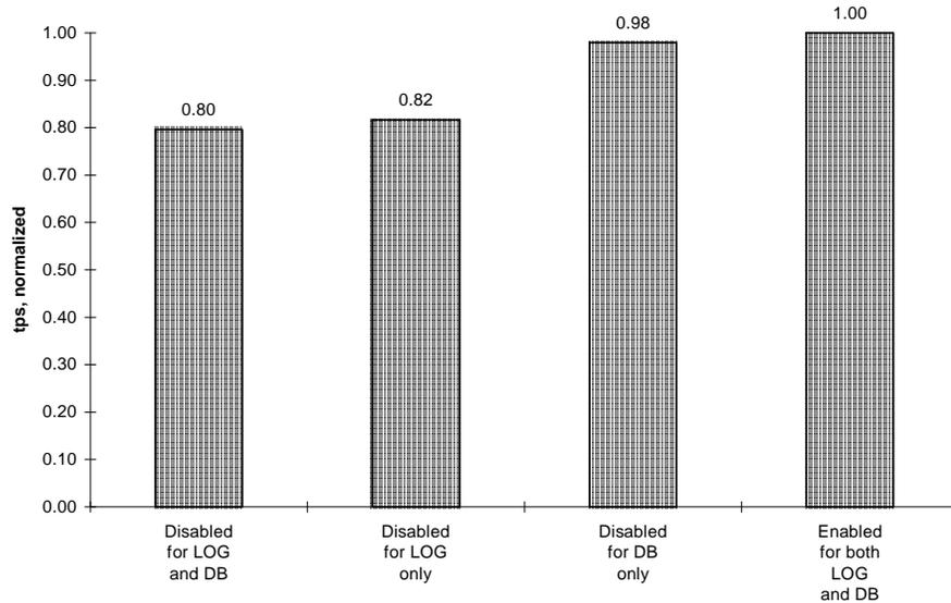
Figure 2-2. Effect of Disabling SMART Array Accelerator
