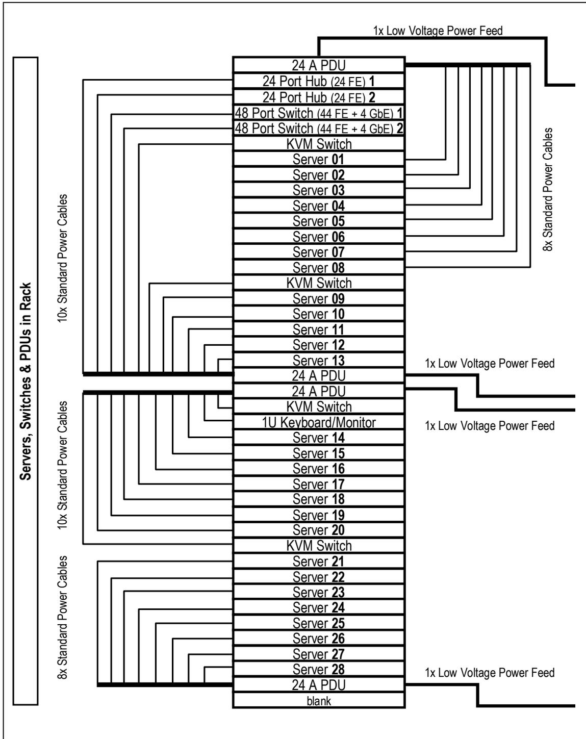
Figure 7. Configuration C (Traditionalist) Power Diagram
