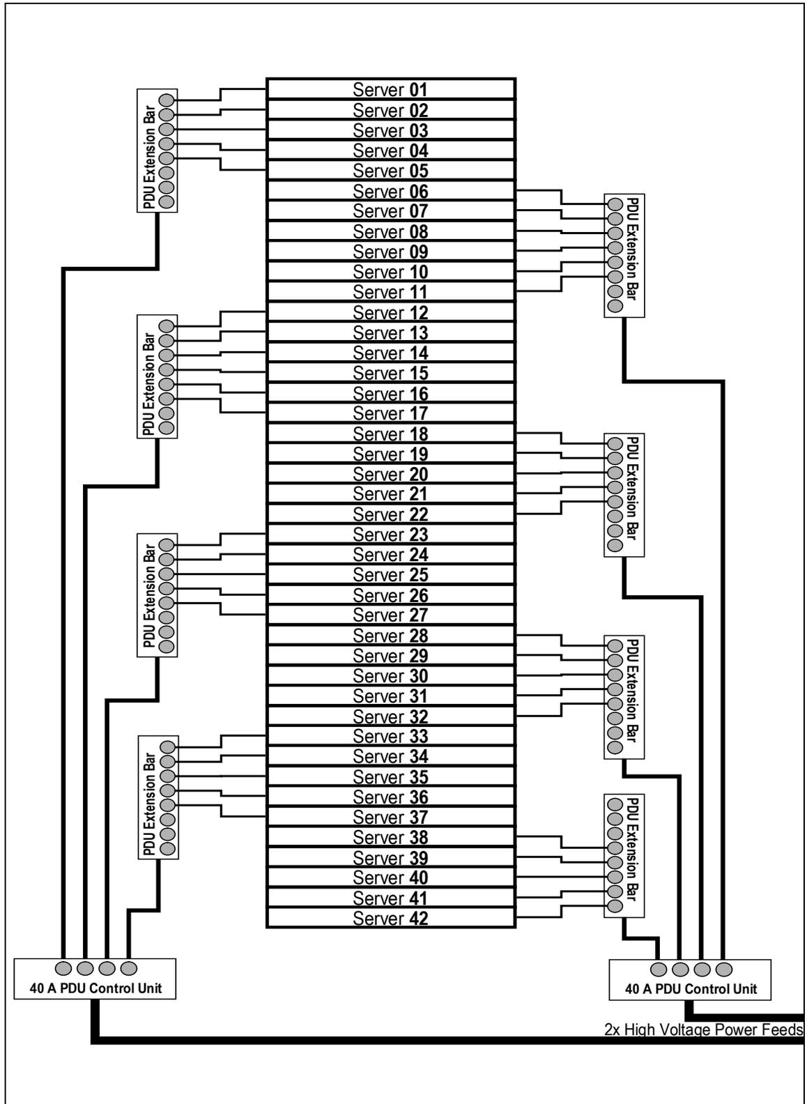
Figure 2. Configuration A (Maximum Performance Density) Power Diagram
