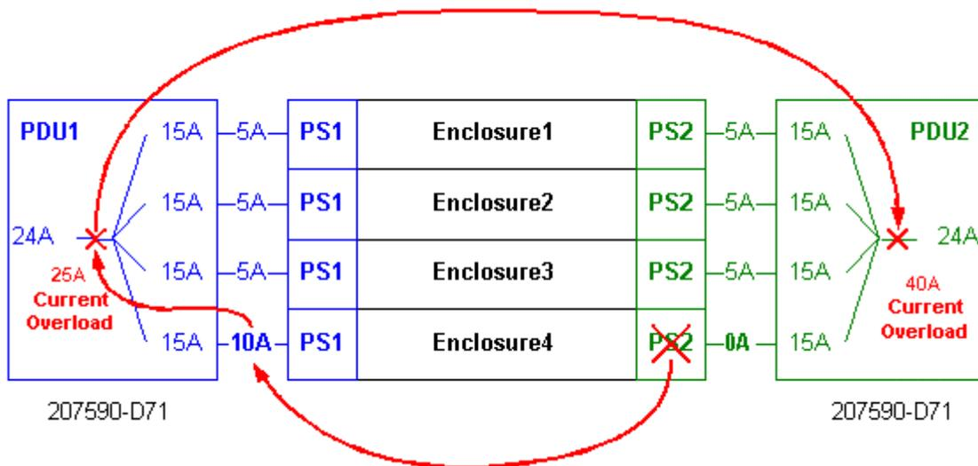
Figure 11. Domino effect caused by low-line current overload
