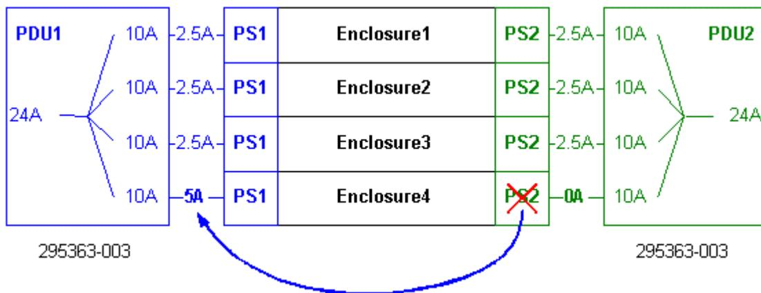
Figure 12. Redundant PDU configuration with four enclosures (high-line)
