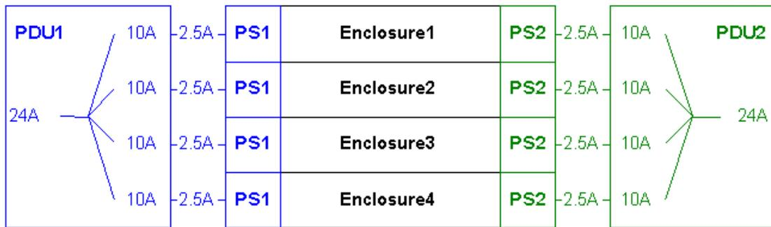
Figure 14. High-line redundant PDU configuration supporting one to four enclosures
