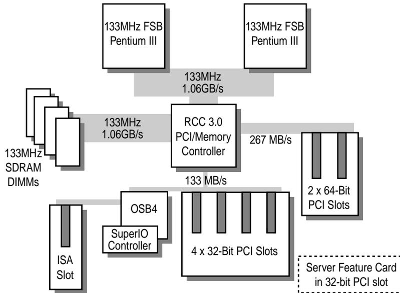
Figure 1. Dual-peer PCI bus architecture in the ProLiant ML350
