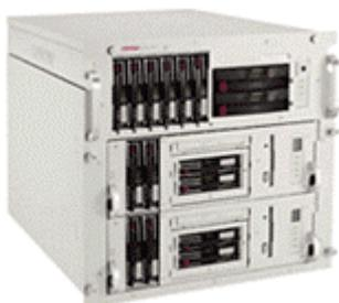
Compaq improved its ProLiant CL1850 Package Cluster with the new ProLiant CL380. Updates include new server capabilities, processors, memories, a PCI expansion slot, and controller module. This uniquely packaged two-node cluster simplifies clustering for business critical applications. It consists of two Compaq server nodes and shared storage pre-packaged in a cost-effective, space-efficient cabinet giving customers the easiest and most affordable clustering solution.
