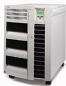
The ProLiant 6000 delivered breakthrough enterprise performance and the highest levels of expansion for the best value in business-critical environments. The ProLiant 6000 offered up to four 500-MHz Pentium III Xeon processors providing industry-leading performance for CPU-intensive applications, such as Windows NT Terminal Server and database applications. The ProLiant 6000 provided leadership performance and unparalleled expansion in an easy-to-service, industry-standard platform.
