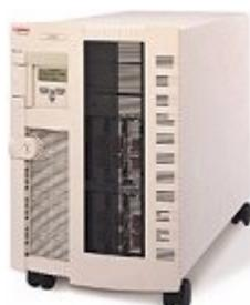
The ProLiant 5500 Server supports up to four 550- or 500-MHz Pentium III Xeon processors with 100-MHz front-side bus and full-speed cache. The 5500 ships with 512-K or 1-MB L2 cache with 2 MB optional. The dual-peer PCI architecture eliminates the need to balance I/O. The system ships with 256 MB of ECC EDO memory expandable to 4 GB using industry-standard DIMMs. The system supplies seven expansion slots, including six PCI and one shared PCI/ISA slot.
