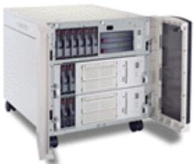
The ProLiant CL1850 includes two 550-MHz Intel Pentium III processors on each server, up to 1-GB SDRAM memory per server, high performance 10,000-rpm SCSI disks, four PCI expansion slots, and up to 252 GB of high performance SCSI storage.
