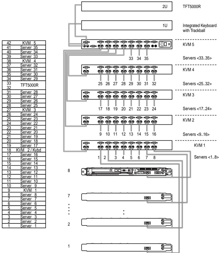
Figure 10: Typical KVM and cascading console switch solution for 35 Compaq ProLiant DL360 Servers
