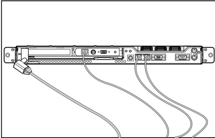
**Figure 8: Typical cabling using the Remote Insight Lights-Out Edition**
