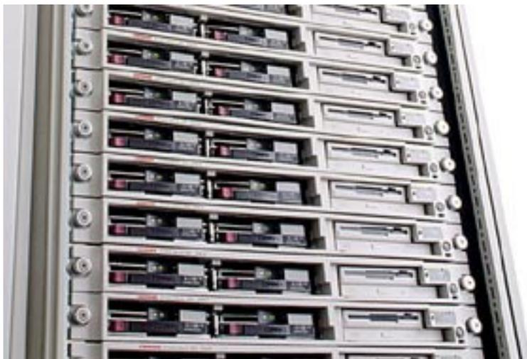
Figure 1: Deployment of 1U ProLiant DL360 ultra-dense servers in a cabinet rack
