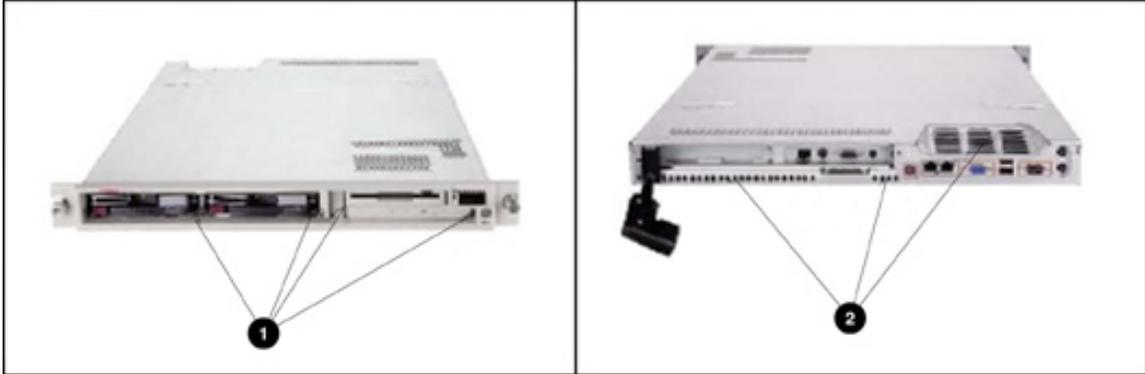
**Figure 5: Intake and Exhaust vents for the Compaq ProLiant DL360 server**
