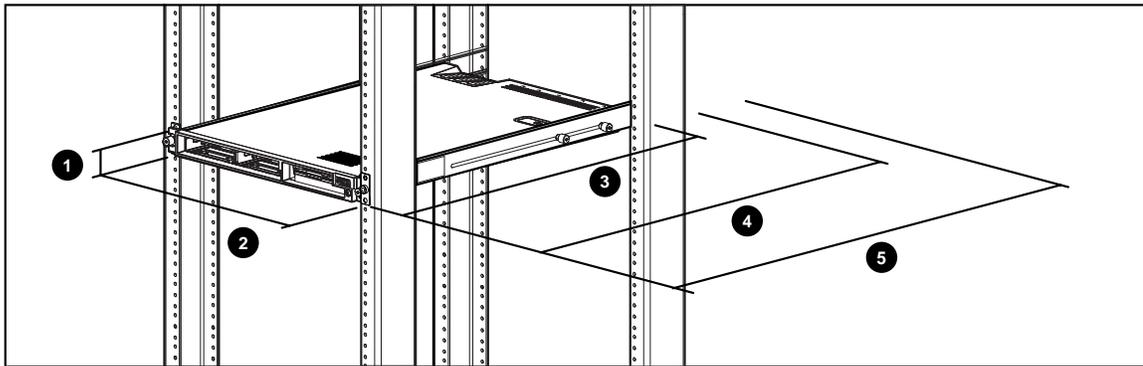
**Figure 4: Height, width, and depth requirements for Compaq ProLiant DL360 server installation using the Compaq Third-Party Rack Option Kit**
