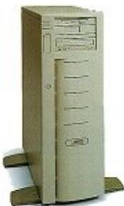
This affordable, mission-critical server was intended for departmental file and application services. FlexSMP System Architecture allowed the ProLiant 1500 to upgrade to dual processing and a 6/200 FlexSMP Dual Processor Board option expanded to a second 200-MHz Pentium Pro processor. The 512-KB secondary write-back cache provided enhanced system performance. The 32 MB of ECC memory was located on the processor board was expandable up to 256 MB.
