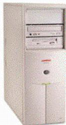
This server joins either the Intel Pentium II Xeon or Intel Pentium III Xeon processor with a 100-MHz GTL+ front side bus and an integrated Wide Ultra2 SCSI Controller offering performance suited for a variety of applications. The affordable ProLiant 400 comes standard with 64-MB, 100-MHz unregistered ECC SDRAM DIMM memory (upgradable to a maximum of 768 MB), an internal mass storage capacity of 54.6 GB, and a high performance 32X Max IDE CD-ROM drive.
