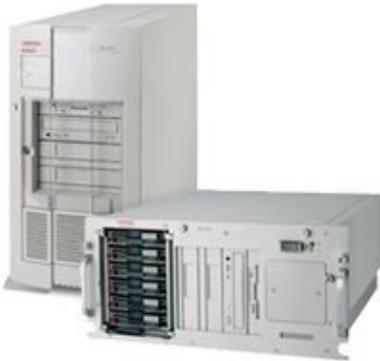
Additional features include dual-peer PCI bus architecture for access to high bandwidth 64-bit/33-MHz PCI slots, optional Integrated Smart Array Controller for additional performance and availability, ten bays to support web hosting, mail, file/print, or small database applications without functionality tradeoffs, and optional Remote Insight Lights-Out Edition for full virtual presence from any remote site.
