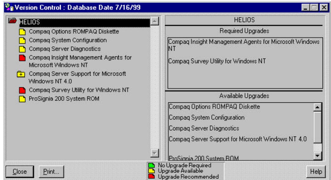
Figure 9 - Compaq Insight Manager shows the software resident on the Integration Server along with updates available from Compaq; you can download updates via the Internet, via a modem connection or from a local CD.
