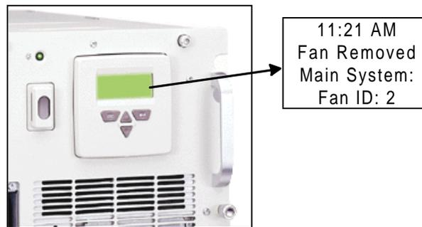
Figure 12: *Integrated Management Display with sample alert message.*
