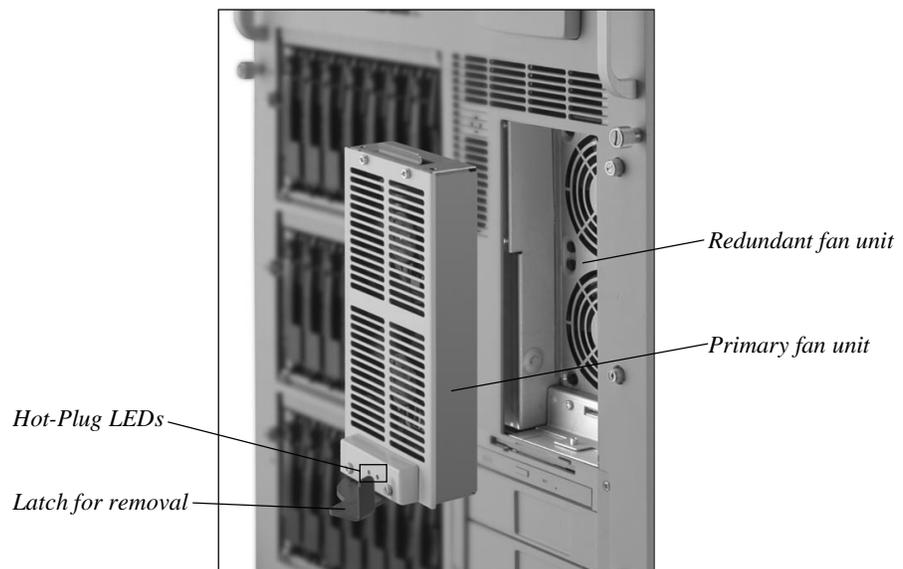
Figure 6: Front hot-plug fans for the processor and memory section of the ProLiant 8000 server.
