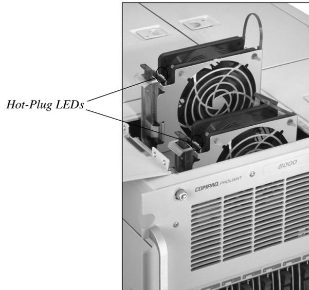
Figure 7: Hot-plug fans for the I/O section in the ProLiant 8000 server.
