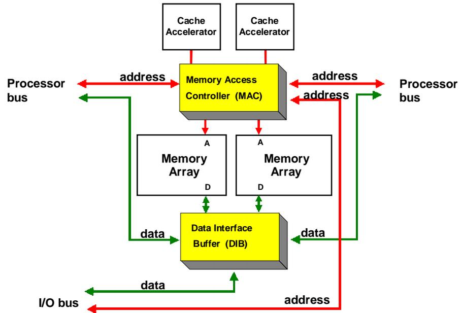
Figure 3: ASIC partitioning in the Profusion chipset.
