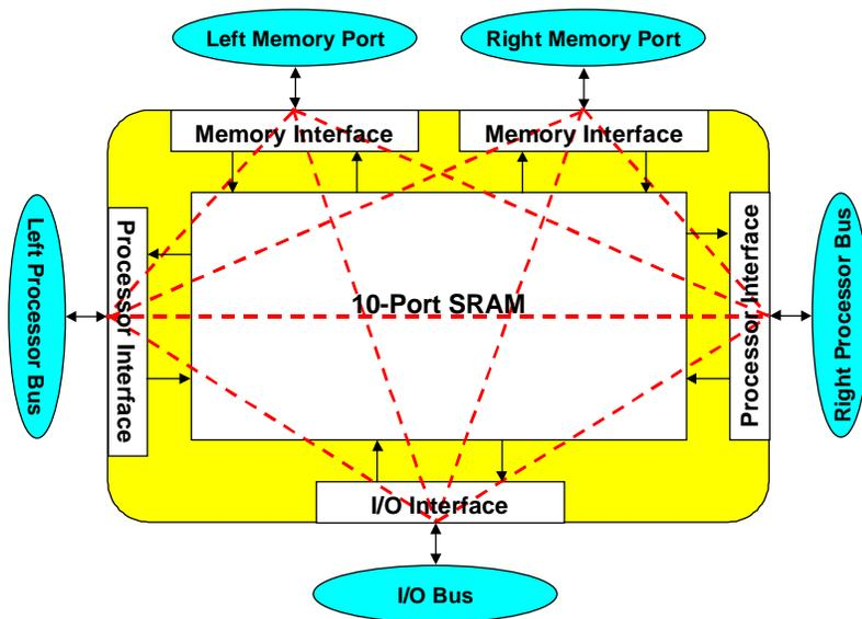
Figure 2: Block diagram of the Profusion crossbar switch.
