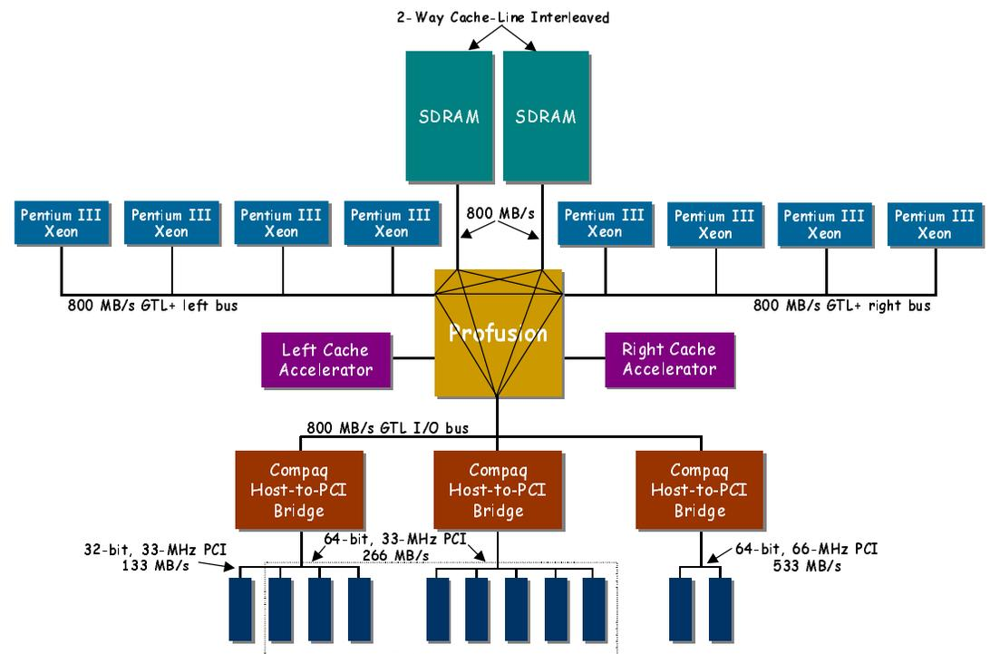
Figure 1: Block diagram of the ProLiant 8000 system architecture.
