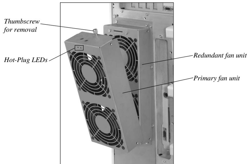
Figure 5: Rear hot-plug fans for the processor and memory section of the ProLiant 8000 server.
