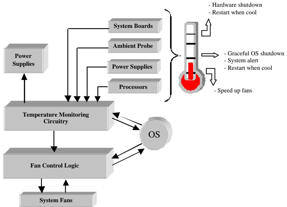
Figure 8: Schematic diagram of fan control logic.
