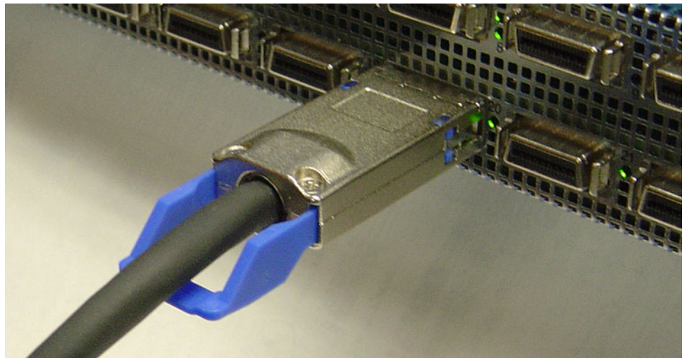
Figure 2-7: Fully Installed InfiniBand Cable with Pull Connector
