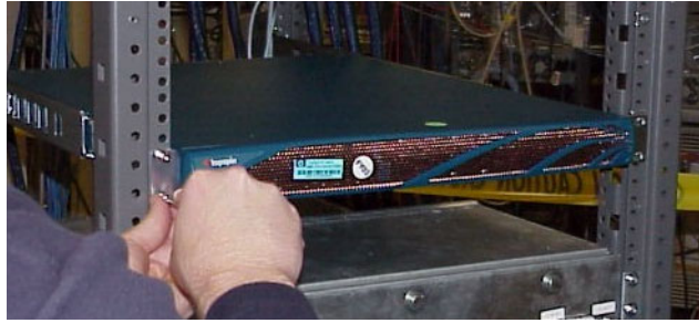
Figure 2-4: Secure the Switch Through the Front Rack Rail
