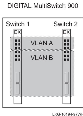
Virtual LANs are a powerful feature of today's switches. They enable a network manager to logically group physically diverse LANs. For example, a LAN on the first floor of an office building can be logically grouped with a LAN on the third floor to form a single virtual LAN. The virtual LAN can then be managed as a unique entity within the network even though the physical components of the VLAN (such as workstations, servers, and so forth) are wired to physically diverse LAN segments.
