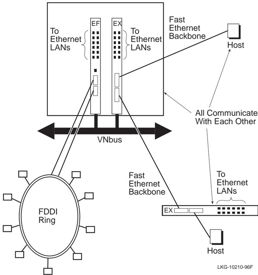
In [Figure 1-16](#), the FDDI LAN attached to the VNswitch 900EF can communicate across the VNbus to the VNswitch 900EX, then over the Fast Ethernet backbone to the Ethernet LANs attached to a remote VNswitch 900EX.
