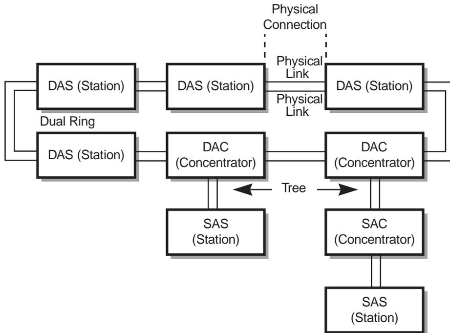
As shown in Figure A-2, all devices connect to each other by means of a full-duplex connection, called a physical connection.
