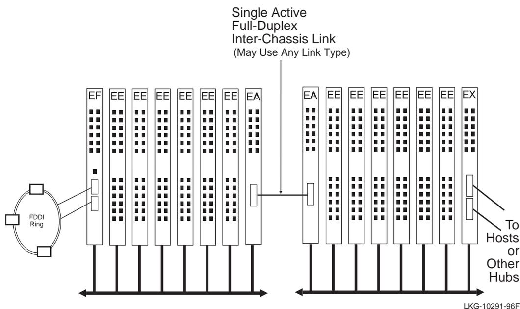
Though not shown in this figure (or in Figure 4-23), more than two parallel links can be configured. For example, two VNswitch 900EA modules could be used in each hub to provide full-duplex links for multiple VLANs, with a separate bridge tunnel configured for each VLAN. In this case (using VNswitch 900EA modules), the dual full-duplex links would provide approximately 620 Mb/s of inter-chassis capacity (155 Mb/s in each direction per link).
