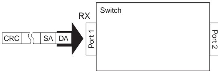
Stage 2 - Receive Complete Frame, Verify Frame Integrity
