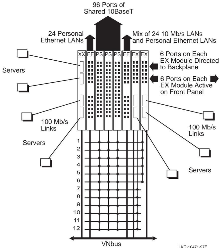
The VNswitch modules in this example are connected to a single **VNbus**, allowing traffic between the VNswitch modules to flow at 400 Mb/s, while also allowing VLANs to span across the modules.
