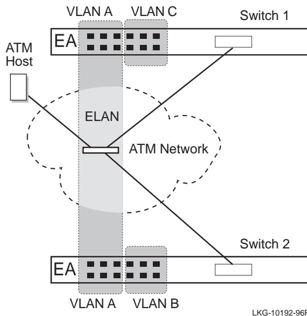
As many as 16 emulated LANs (ELANs) are supported on each VNswitch 900EA, XA, and FA module. Each ELAN may consist of VLANs that span multiple modules in the hub, allowing LANs from the VNswitch 900EE, EX, XX, or EF to be joined with LANs on other VNswitch modules residing in a separate hub on the other side of an ATM network. Refer to Figure 1-19.
