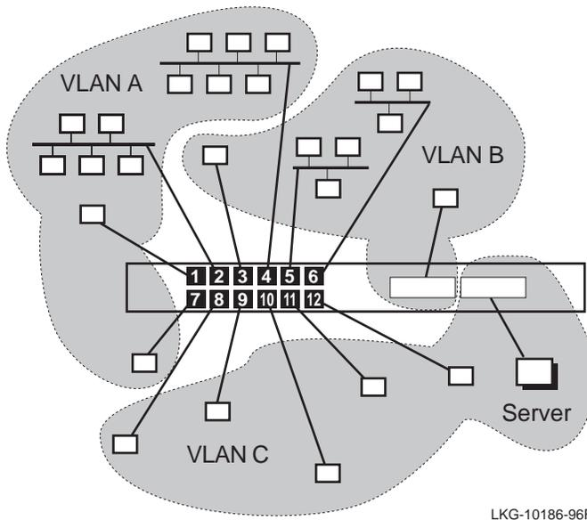
As shown in [Figure 1-14](#), the LAN attached to port 2 has been grouped with the LAN attached to port 4, along with the personal Ethernet LANs attached to ports 1 and 7. These four LANs form a single VLAN (VLAN A). LANs attached to ports 3, 5, and 6 are grouped with one of the Fast Ethernet ports to form another VLAN (VLAN B). The personal Ethernet LANs attached to ports 8 through 12, along with the other Fast Ethernet port, are grouped into VLAN C.
