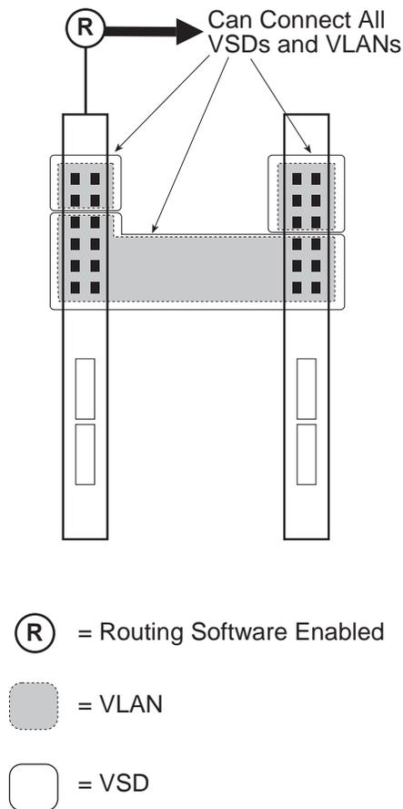
As shown in [Figure 3-39](#), a module with its routing software enabled allows traffic to be routed between VSDs and VLANs. Without the routing software enabled, no traffic can flow between VSDs or VLANs.
