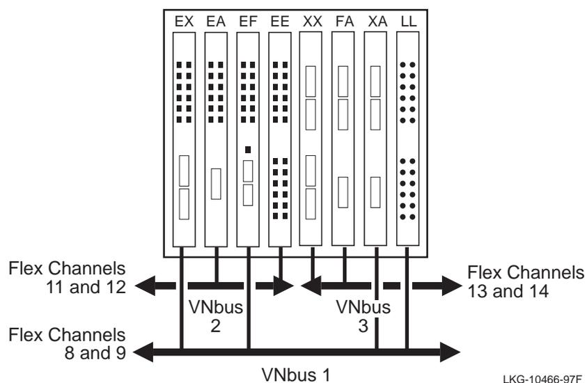
As shown in [Figure 3-8](#), three distinct VNbuses are supported. The VNbuses are physically isolated from each other and each forms a separate network.
