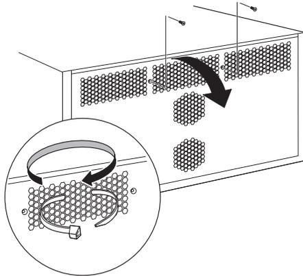
**Note:** Using a tie wrap (instead of a solid object like a screwdriver) prevents damage to the back panel.
