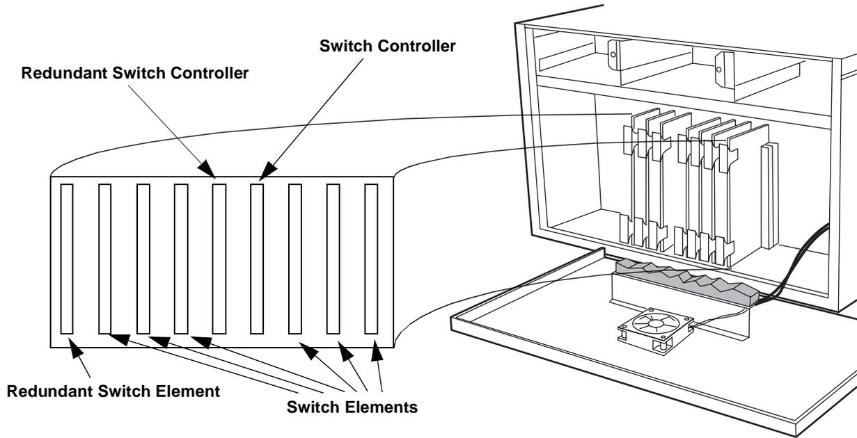
4 Insert the module into the selected slot. The slots are keyed to ensure proper insertion.
