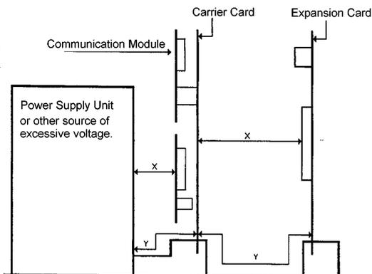
Except for the edge connector which plugs into the host's expansion slot, clearance distance (Xmm) and creepage distance (Ymm) as given in the above table, must be maintained between the communication card and any other assemblies which use or generate a hazardous voltage.
